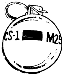
ABC-M25A2, CS riot control hand grenade. Color/markings: gray, red band(s) and red printing.
